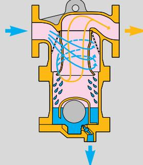
**1** Fluid enters the inlet of the separator, and a complex series of fins changes the steam or air flow into a high-speed cyclone flow, separating even mist-like condensate.
