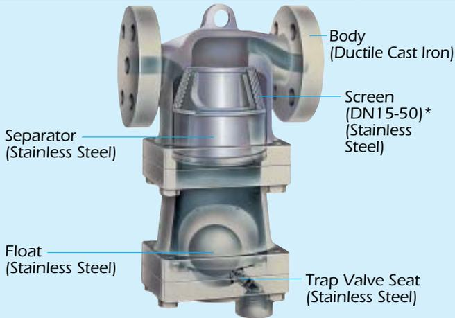
\* Screen for sizes DN 65-100 is in Trap Cover
